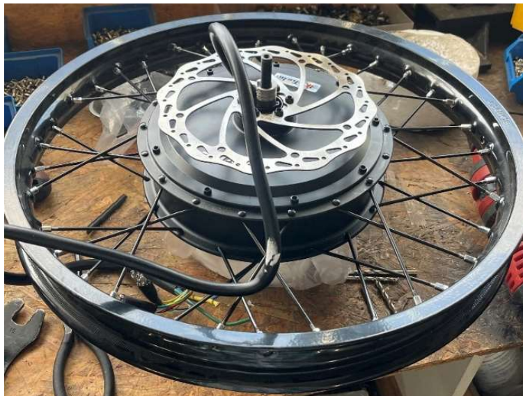
Figura 33 – Motor Mxus 3k turbo 3kW.
